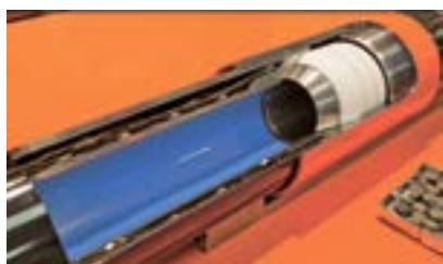
Базовая конструкция ТЛТ Basic construction of the insulated lift pipe
